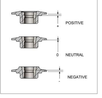
The standard height Crane Cams valve stem lock part numbers are listed with each diameter valve stem (where applicable) to achieve these figures. Remember, most of our valve stem locks are also available in +.050" and -.050" heights (see pages 360-361), to extend the available height combinations that can be created.
