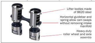
valve spring seat pressures up to 240 lbs. (closed) for drag racing and 220 lbs. for sustained oval track competition. The lifter bodies are machined from 8620 steel and feature both horizontal and vertical guide bar designs. An added benefit of the spring-loaded horizontal guidebar setup is the ability to change cams without intake manifold removal (providing a "rev kit" is not used)—great for dyno and ontrack testing.
